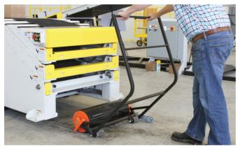
Access for maintenance is designed with safety and speed involved. Heavy drive motors are accessed with a maintenance tool, making changes faster, safer and reducing downtime.
