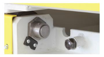
Reliable performance starts with high capacity weight bearing roller bearings and cam followers that support all the booms during movement and at full extension, for increased reliability. Field adjustability for precision installations helps improve reliability.
