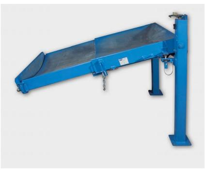
The Tip Chute is designed to assist the loading of cargo into delivery trucks. It spans the gap from the feeding conveyor / roller section to the delivery truck. The Tip Chute rotates to the lowered position and the discharge door extends to 5'6" from the stored position.
